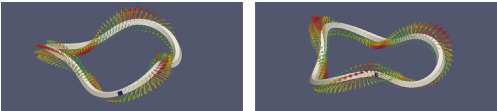
FIGURE 5. Snapshots of ring taken 1/2 of a temporal period apart. The material patch on the surface, visible in each frame, demonstrates that the motion is not a rigid-body rotation of the helix about its axis. The force vectors are also depicted along the surface, with the colours indicating magnitude.
