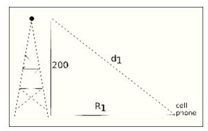
**Fig. 4** This schematic shows a 200 m tower with a receiver at the top. The distance to the cell phone recorded by the tower is  $d_1$ . The distance from the phone to the base of the tower is  $R_1$ .
