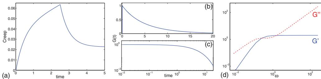
FIG. 11. Stokes-Maxwell element with  $E = 1$ ,  $\eta = 5$ ,  $\ell(0) = 1$ ,  $\varepsilon_0 = 0.1$ ;  $\mu_e = 1$  and  $\delta = 1/4\pi$  and an initial length 1: (a) creep function with  $\sigma_0 = 0.05$ , (b) relaxation modulus and (c) its log-log plot, (d) storage and loss moduli.
