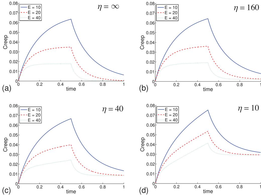
FIG. 13. Creep functions for the link-node system attached to the wall subject to the step-function shear stress Eq. (1) with  $\sigma_0 = 1$ ,  $t_0 = 0$ , and  $t_1 = 0.5$  with stiffness  $E = 10$ ,  $E = 20$ ,  $E = 40$ , respectively. (a) Response of the Stokes-spring network. (b)–(d) Response of the Stokes-Maxwell networks with damping constants  $\eta = 160$ ,  $\eta = 40$ , and  $\eta = 10$ , respectively. In each case,  $\mu_e = 1$  and  $\delta = 1/4\pi$ .
