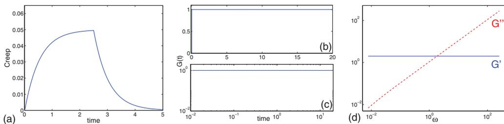
FIG. 8. Stokes-spring element with  $E = 1$ ,  $\ell = 1$ ,  $\varepsilon_0 = 0.1$ ;  $\mu_e = 1$  and  $\delta = 1/4\pi$  and an initial length 1: (a) creep function for  $\|\mathbf{f}\| = 0.05$ , (b) relaxation modulus and (c) its log-log plot, (d) storage and loss moduli.
