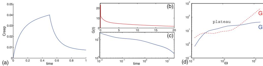
FIG. 19. Double-linked Stokes-Maxwell network based on elements with  $E_{a,b} = 10$ ,  $\eta_a = 10$ , and  $\eta_b = 160$ : (a) creep functions with  $\sigma_0 = 1.0$ , (b) relaxation modulus for  $\varepsilon_0 = 1.0$ , and (c) its log-log plot, (d) storage and loss moduli with solid and dashed line for  $\varepsilon_0 = 0.1$ ,  $\mu_e = 1.0$ , and  $\delta = 1/4\pi$  in all tests.
