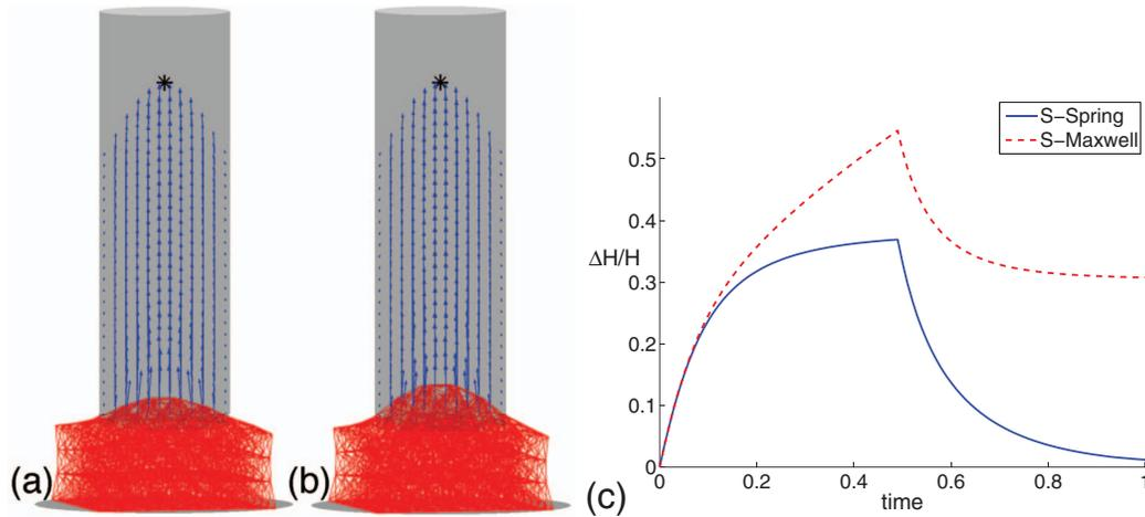
FIG. 20. Micropipette aspiration simulations at the sample mesh, links stiffness  $E = 10$  and viscosity  $\eta = 5$ . Micropipette aspiration simulation with velocity field at time  $t = 0.5$  for (a) Stokes-spring network and (b) Stokes-Maxwell network, respectively. (c) Creep function for the micropipette aspiration on both networks: relative aspiration length vs. time, sink strength 5.
