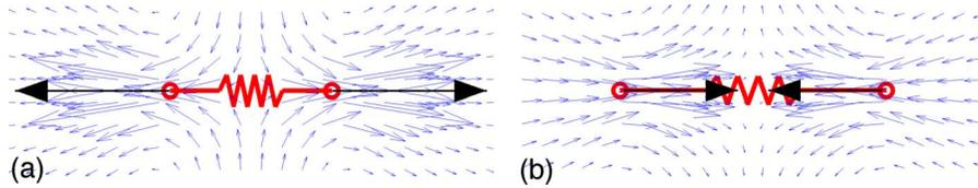
FIG. 7. Acting forces (bold arrows) and velocity field around the Stokes-spring element during a creep test, (a) at  $t_0$  and (b) at  $t_1$ , the beginning of loading and unloading phase of the test, respectively.
