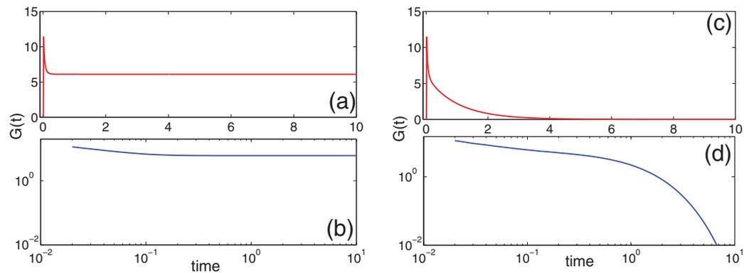
FIG. 14. (a) Relaxation modulus for the Stokes-spring network, (b) its log-log plot, (c) relaxation modulus for the Stokes-Maxwell network, (d) its log-log plot. Here,  $E = 10$ ,  $\eta = 10$ ,  $\varepsilon_0 = h = 1$ ,  $\mu_e = 1$ ,  $\delta = 1/4\pi$ .
