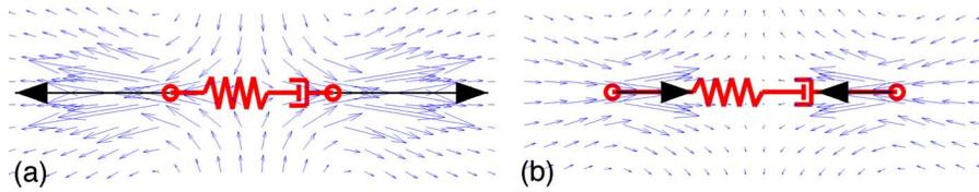
FIG. 10. Acting forces (bold arrows) and velocity field around the Stokes-Maxwell element during a creep test, (a) at  $t_0$  and (b) at  $t_1$ , the beginning of loading and unloading phase of the test, respectively.
