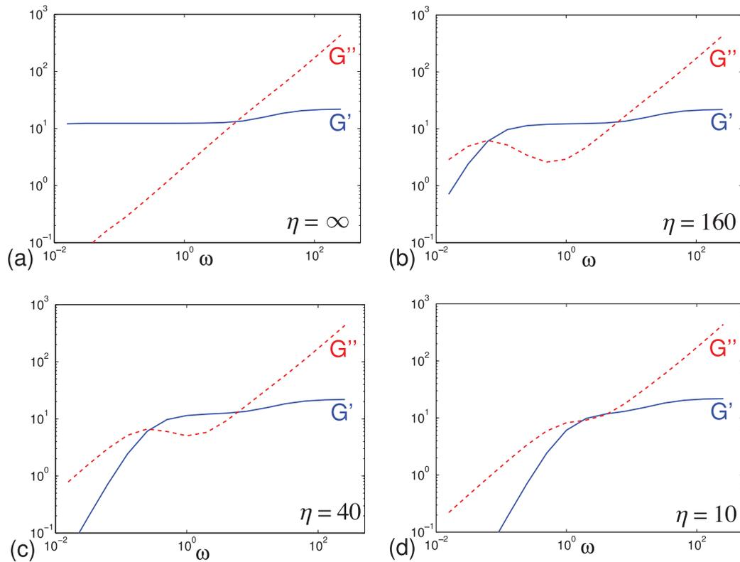
FIG. 16. Log-log plot of  $\omega$  vs. the storage and loss moduli for the shearing sinusoidal strain, Eq. (3) with the amplitude  $\varepsilon_0 = 0.1$ , a stiffness constant for each element in the network is fixed at  $E = 10$ . (a) Moduli for the Stokes-spring network. (b)–(d) Moduli for the Stokes-Maxwell network: damping constant  $\eta = 160$ ,  $\eta = 40$ , and  $\eta = 10$ , respectively. In each case, we use  $\mu_e = 1$  and  $\delta = 1/4\pi$ .
