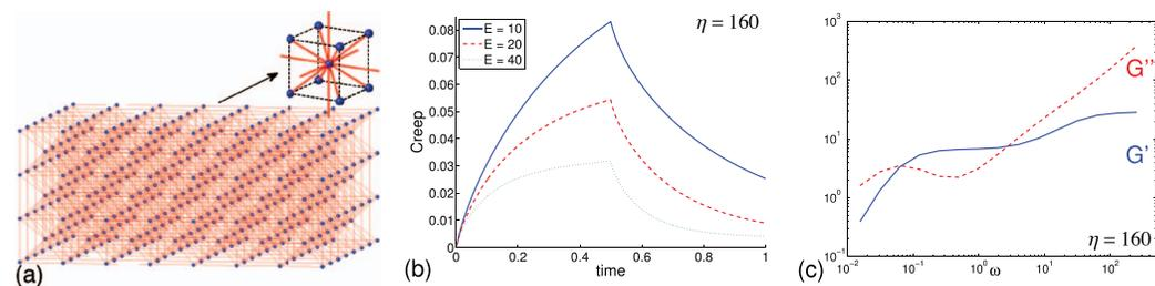
FIG. 17. (a) Viscoelastic link-node system of the body-centered cubic topology, (b) creep functions for the Stokes-Maxwell system with damping constants  $\eta = 160$  and with stiffness  $E = 10$ ,  $E = 20$ ,  $E = 40$ , respectively, (c) storage and loss moduli for the system with  $E = 10$ ,  $\mu_e = 1$ , and  $\delta = 1/4\pi$ .
